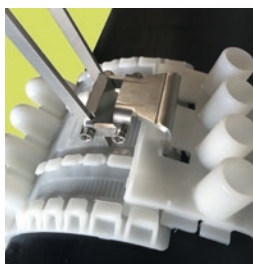
Applying a collar F.
